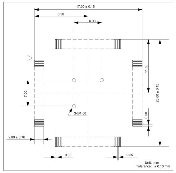
Figure 6 Recommended Dimensions for Mount Pad
